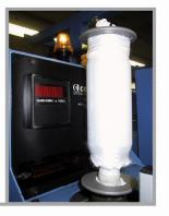
We ran the coverings test on Menegatto machines type 1500 at 22,000 RPM, with 256 positions on 13/7 dtex D.C. -1,750 tpm. flat Nylon on Lycra 44 dtex.
